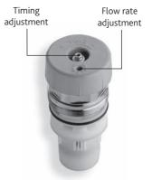
It is possible to progressively vary the timing and flow rate without removing the cartridge from the tap body using a 2mm hexagonal wrench.
