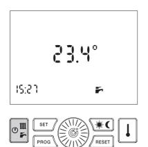
**Press 3 Times - WINTER:** the heat interface unit is enabled to produce both domestic hot water and spece heating.
