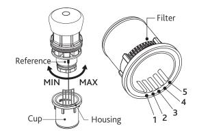
The flow rate depends on the position of the reference (located on the cartridge body) in the seat of the plastic cup.
