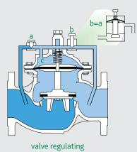
The 2-way control system provides sensitive, accurate and constant modulation of the main control valve.
