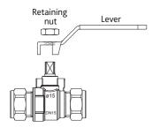
Fully open the valve so that the position of the valve and lever are known.
