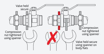
Further tighten the compression nut as per the following recommendation.
