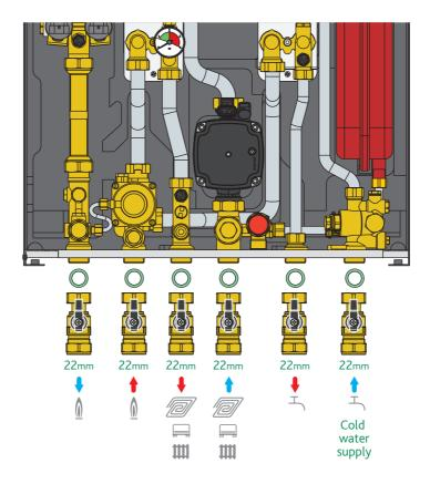
Fit the ball valves to the HIU as shown, noting the duty of each connection.
