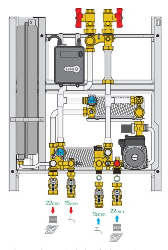
Fit the ball valves to the HIU as shown, noting the duty of each connection.
