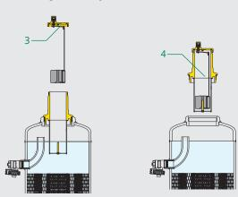
The components that control the air venting are accessed by removing the cover (3).
