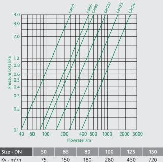
The maximum recommended flow velocity inside the pipe is 1.2 m/s. The following shows the maximum flow rates to meet this
