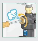
When necessary, it is possible to use the manual air vent in the cap to expel air from inside the strainer.
