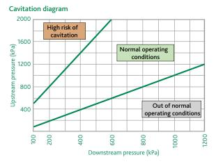
In order to minimise the risk of cavitation in the reducing valve, which could cause malfunctions with the risk of erosion in the seal area, vibration and noise, you are strongly advised to refer to the operating conditions specified in the diagram.
