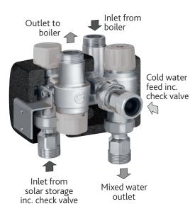
The valve should be installed with isolation valves, strainers and check valves at the water inlets.
