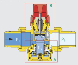
Device A regulates  $\Delta p_i (p_2 - p_3)$  and keeps it constant across the valve B by means of an automatic action (balancing between the force generated by the differential pressure and the internal opposing spring).
