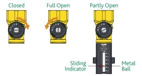
To regulate the flow, firstly with the aid of the sliding indicator, mark the reference flow rate to which the valve requires setting.
