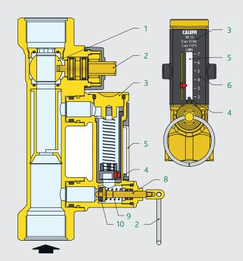
The valve regulates using the ball (1), operated by the control stem (2)
