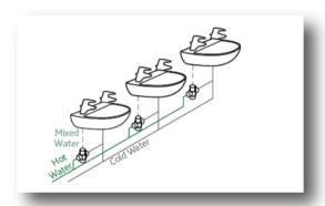
As the name suggests a point of use mixing valve is designed to be installed to a single outlet, or in some instances back to back sinks providing the run of pipe is no longer than 2m.
