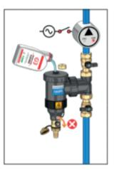
Allow to circulate through the system for 1 hour. Stop the circulator and drain the circuit until clean water comes out.
