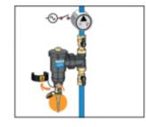
Close the shut-off ball valves and fill with C1 - INHIBITOR via the dirt separator.
