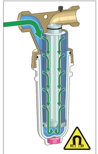
3) The water passes through the centre of the cartridge and comes into contact with the internal elements (Cu alloy - Zn/Ti), where the battery effect and whirling motion cause the first aragonite crystals to form.
