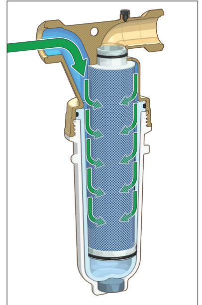
2) The water is channelled towards bottom of the device, where the magnet is located. The magnet, which does not come into direct contact with the water, captures and retains the ferromagnetic impurities and helps to improve the efficiency of the device. The flow is reversed at the bottom and all the water is therefore channelled into the cartridge.
