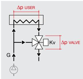
In these two types of circuit, the two- or three-way diverter valve regulates the flow rate passing through the user circuit. In such cases, it is important to have good authority by dimensioning the regulating valve to ensure that the pressure drop is not too low compared to that of the user circuit. Recommended values for rapid sizing can be chosen considering:
