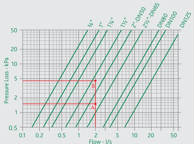
Using the 610 series flow chart, with a flow rate of 2 l/s, moving up vertically the A and B points are identified, which are obtained at the intersection with the respective pressure loss values.
