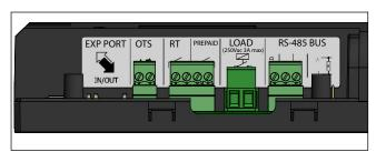
All the terminals are mounted on removable connectors to facilitate wiring operations.
