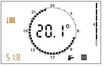
Heating flow probe temperature (SATK2210. - SATK2220.)
