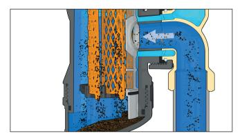
A central magnet captures and retains ferrous impurities down to the smallest sizes.
