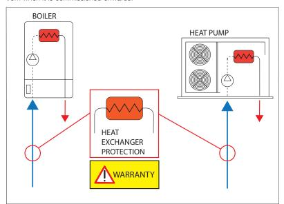
It is therefore necessary to use a device that can remove impurity particles in all working conditions.
