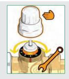
Check the PICV setting by measuring the flow rate passing through the terminal unit using the integral Venturi. See section "Flow rate measurement".
