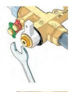
Remove the strainer holder cartridge and clean the strainer under running water.
