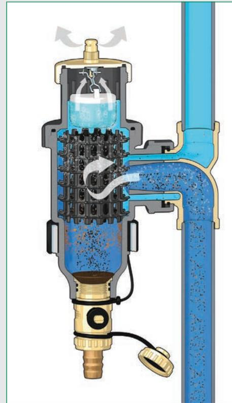
Dirt separators operate by a combination of physical principles. The internal element is constructed to form a radial net shaped element.
