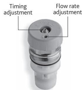
It is possible to progressively vary the timing and flow rate without removing the cartridge from the tap body using a 2mm hexagonal wrench.
